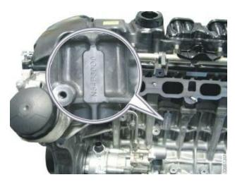
For example, the new N52KP engine which is a variant of the original N52 engine will now be known as the N52B30O1. This would be instead of the traditional "TU" suffix as in - N52B30TU.
