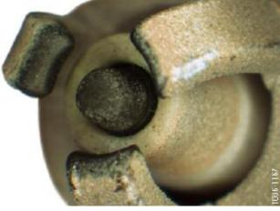
The spark plug above shows a normal wear pattern with no excessive electrode wear or insulator damage.
