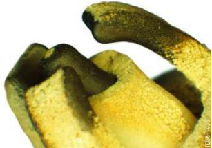
The spark plug above shows erosion of the electrode on one side which could be an indication of fuel spray "diversion".
