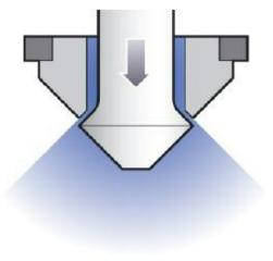
The spray cone (1) of a piezo-injector can diverge during operation (2). Due to the formation of soot inside the engine, such divergence is perfectly normal and acceptable to a certain extent. If, however, spray divergence reaches the stage where it begins to spray the spark plug wet, the spark plug may incur damage.
